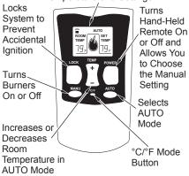
Figure 48 - Thermostat Hand-Held Remote Control Unit HRC200
